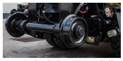
As option available: Friction Drive System available for 1404 ZW-CR with track width 1000 mm.
